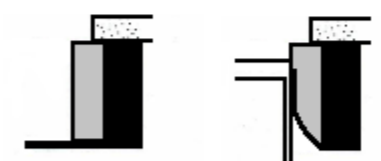
SHELTER CURTAINS CURVE AROUND SIDES OF TRAILER AND BOTTOM PADS FILL THE GAPS
